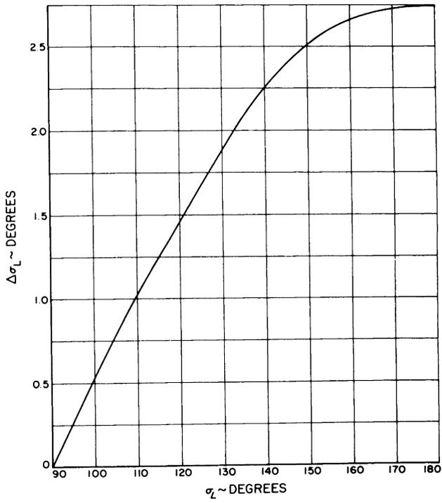
Fig. 7 Effect of Earth rotation upon firing azimuth
