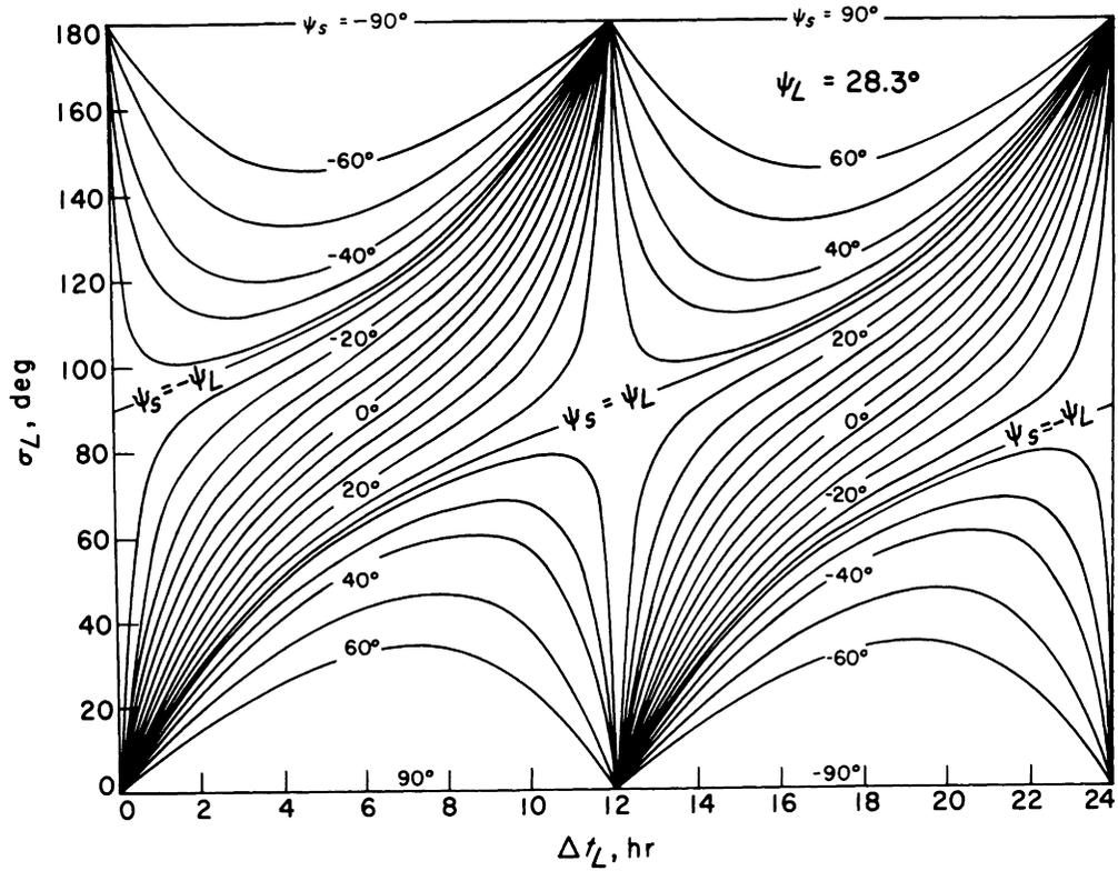
Fig. 5 Firing azimuth vs. launch time for symmetric situation
