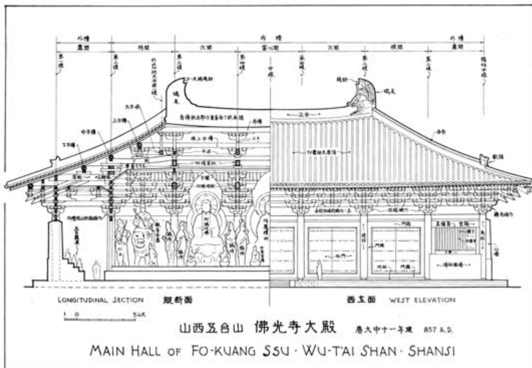
FIGURE 1.1a. Section and elevation of the Great Buddha Hall, Foguang Monastery, Mount Wutai. 857 CE. From Liang, A Pictorial History of Chinese Architecture , fig. 24j. Diagram courtesy of Lin Zhu.
