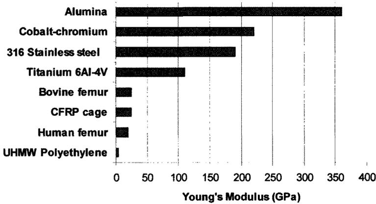
Figure 5 Modulus of elasticity of implant materials. (Courtesy of H. Serhan, DePuy AcroMed Corp.)
