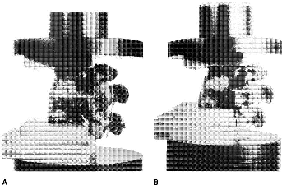
**Figure 4** CFRP cage construct subject to compression testing: (A) before compression; (B) after compression failure. (From Ref. 21.)
