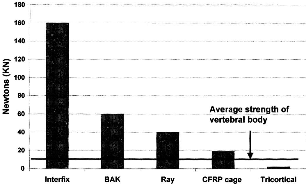
**Figure 2** Static compressive strength of cages versus allograft. (Courtesy of H. Serhan, DePuy AcroMed Corp.)
