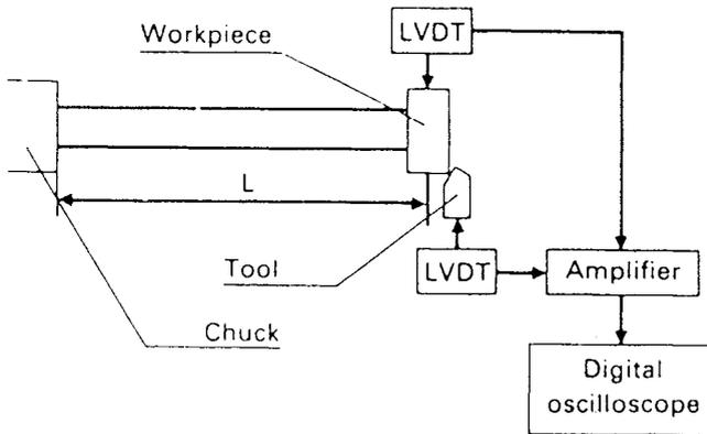
**Figure 1.7** Cantilever workpiece for measuring cutting process stiffness and measurement setup.
