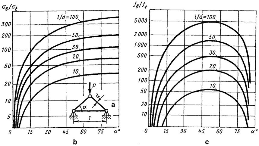
**Figure 2.5** Ratios of (b) stresses and (c) deflections between (a) a double-supported beam in Fig. 2.4a and a truss bridge in Fig. 2.4b.
