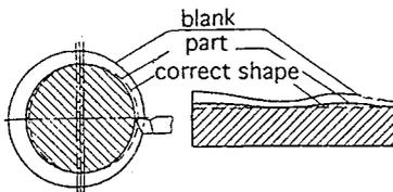
**Figure 1.5** Evolution of geometry of machined parts when machining system has finite stiffness.
