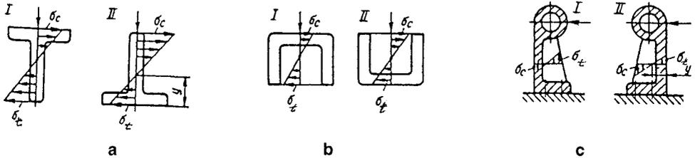
**Figure 2.8** Increasing compressive stresses at the expense of tensile stresses.
