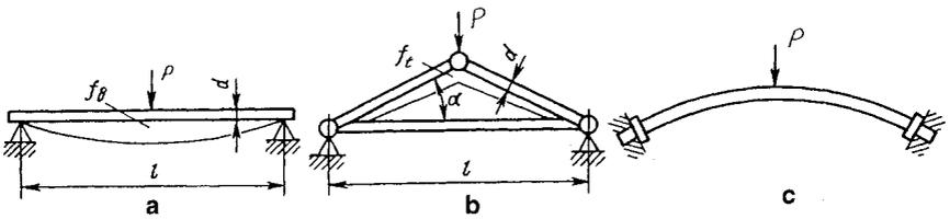
**Figure 2.4** Typical load-carrying structures: (a) double-supported beam; (b) truss bridge; (c) arch.
