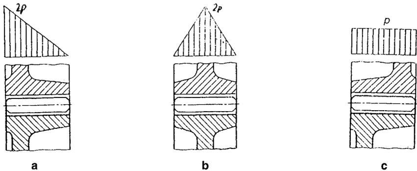
**Figure 1.1** Contact pressure distribution in meshing gears as influenced by design of gears.
