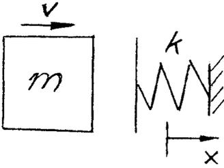
**Figure 1.4** Impact interaction between moving mass and stationary spring.
