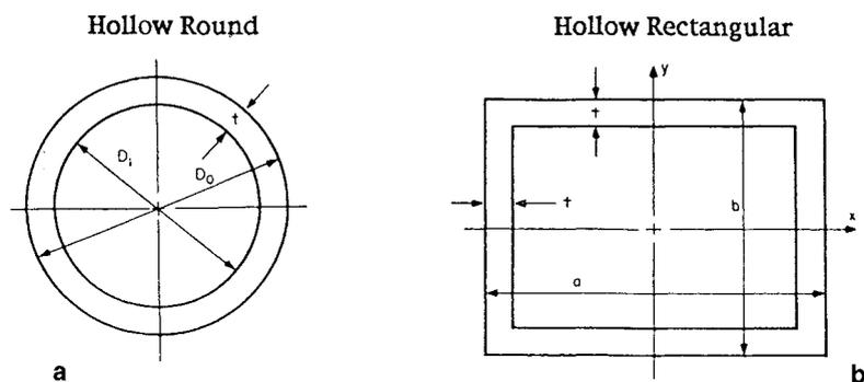
**Figure 2.12** Typical cross sections of a manipulator link: (a) hollow round (ring-like); (b) hollow rectangular.
