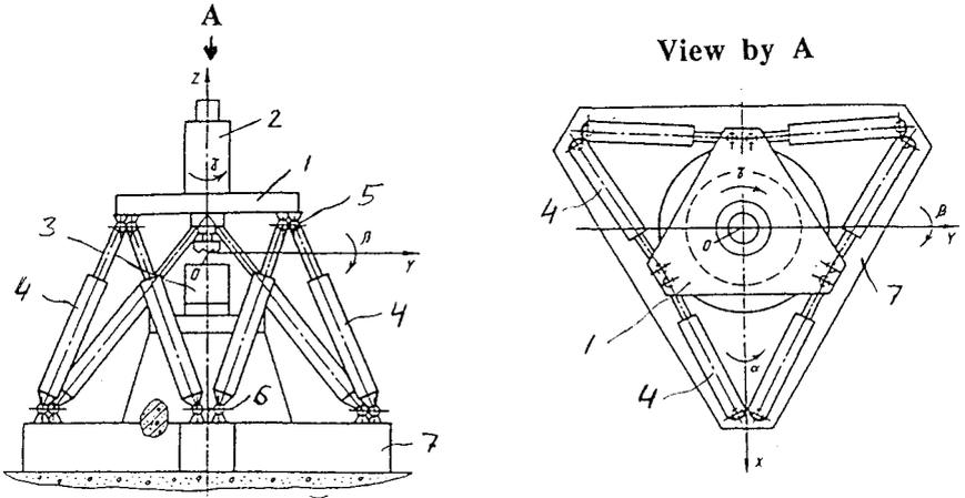
**Figure 2.9** Design schematic and coordinate axes of Russian machining center based on the Stewart Platform kinematics.
