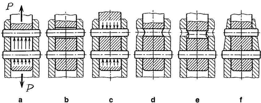
**Figure 1.3** Influence of component deformations on load distribution.
