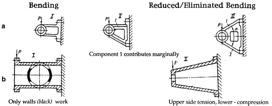
**Figure 2.6** Use of tension/compression instead of bending for structural components.
