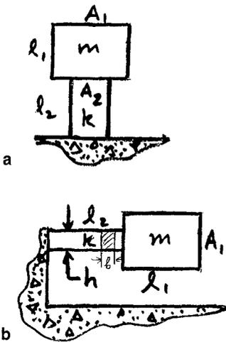
**Figure 1.9** (a) Tension-compression and (b) bending single degree of freedom vibratory systems.
