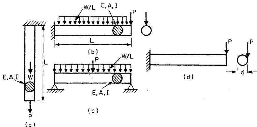
**Figure 2.1** Various modes of loading of a rod-like structure: (a) tension; (b) bending in a cantilever mode; (c) bending in a double-supported mode; and (d) bending with an out-of-center load.
