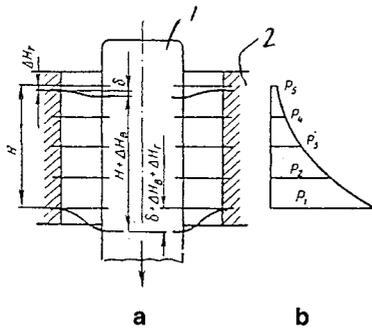
**Figure 1.2** Contact pressure distribution (b) in threaded connection (a).
