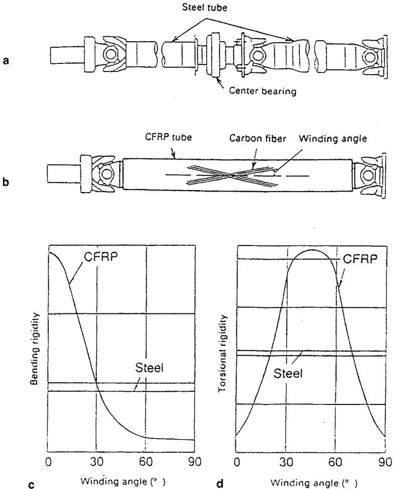
**Figure 1.10** (a) Steel and (b) composite propeller shafts for automotive transmissions and comparison of their (c) bending and (d) torsional rigidity.
