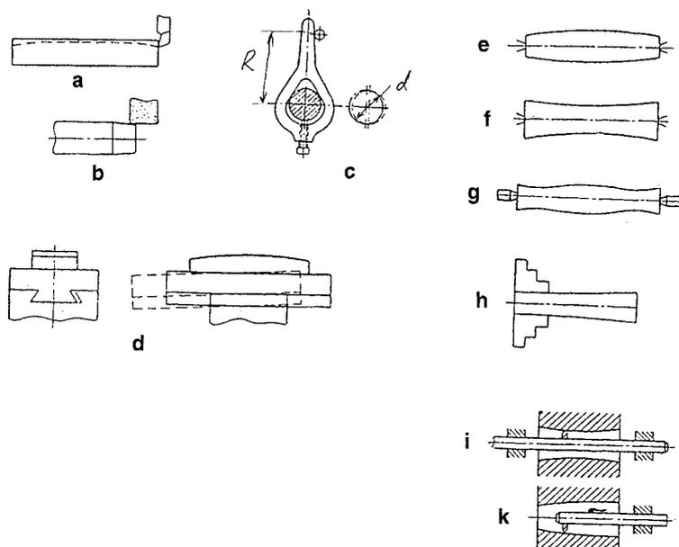
**Figure 1.6** Influence of compliances in the machining system on geometry of machined parts.
