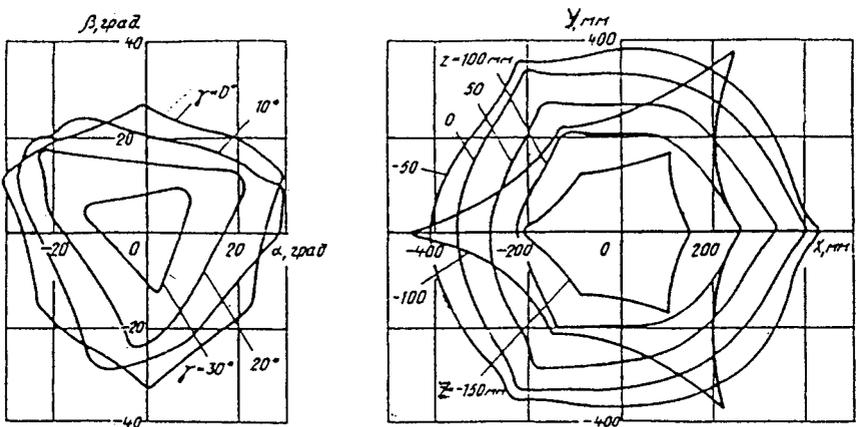
**Figure 2.10** Work zone of machining center in Fig. 2.9.
