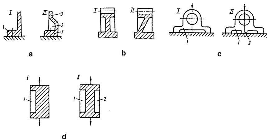
**Figure 2.7** Reduction of bending deformations in structural components.
