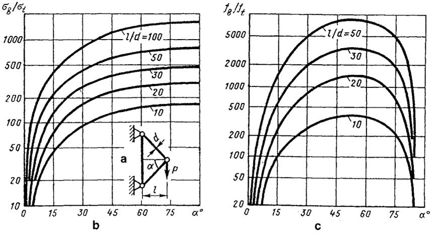
**Figure 2.3** Ratios of (b) stresses and (c) deflections between a cantilever beam (diameter  $d$ , length  $l$ ) and (a) a truss bracket.
