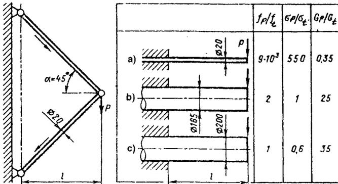
**Figure 2.2** Comparison of structural characteristics of a truss bracket and cantilever beams.
