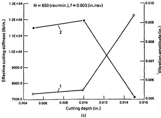
**Figure 1.8** Effective cutting stiffness (line 1) and workpiece vibration amplitude (line 2) vs. (a) cutting speed, (b) feed, and (c) depth of cut.
