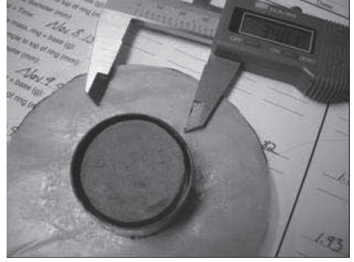
Figure 4. Digital micrometer used for the measurement of the diameter and thickness of shrinkage specimens.
