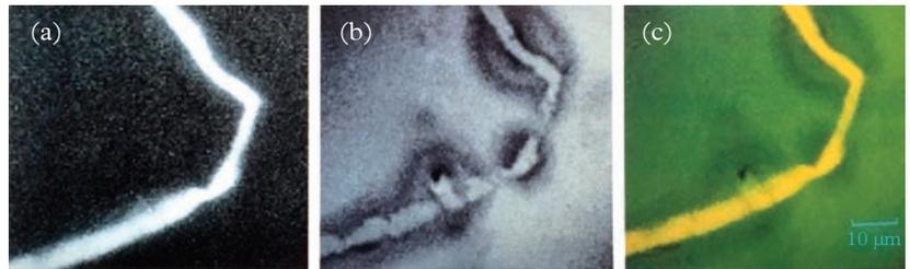
**Figure 1.4.15** SEM compositional maps, using characteristic X-rays, of a Cu–Zn specimen showing diffusion-induced grain boundary migration. (a) Zn-map, with Zn in white, (b) Cu-map, with 90% Cu being black, and (c) a pseudo-color superposition image with Cu in green and Zn in yellow.
