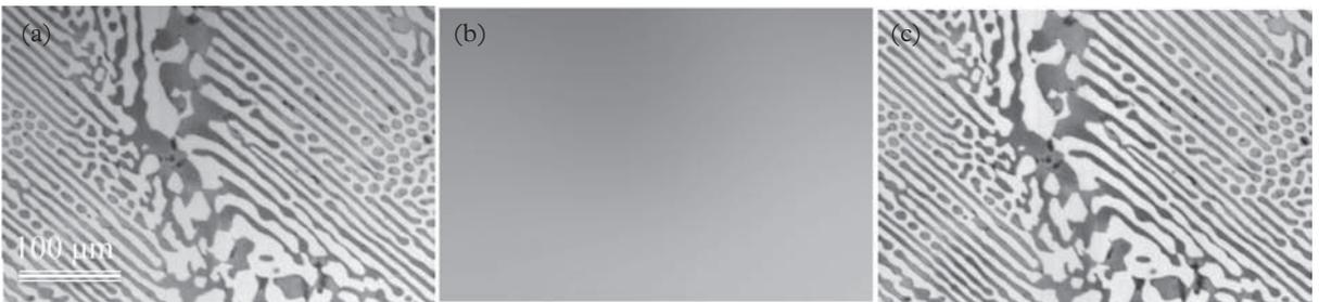
**Figure 1.4.23** Background subtraction. (a) An optical micrograph of hypereutectic cast iron at  $200\times$  BF,  $1300 \times 1030$  pixels that is unevenly illuminated. (b) The estimated background image intensity. (c) The background subtracted image.
