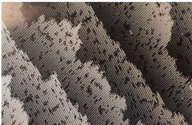
**Figure 1.4.17** Large-scale, atomic resolution, topographical STM image of the Si(100) $2 \times 1$  surface showing two kinds of steps and various point defects. This is technologically most important as integrated circuits are made on this silicon surface and understanding the local structure on the atomic scale is important for processing and manufacturing of semiconductor microprocessors.
