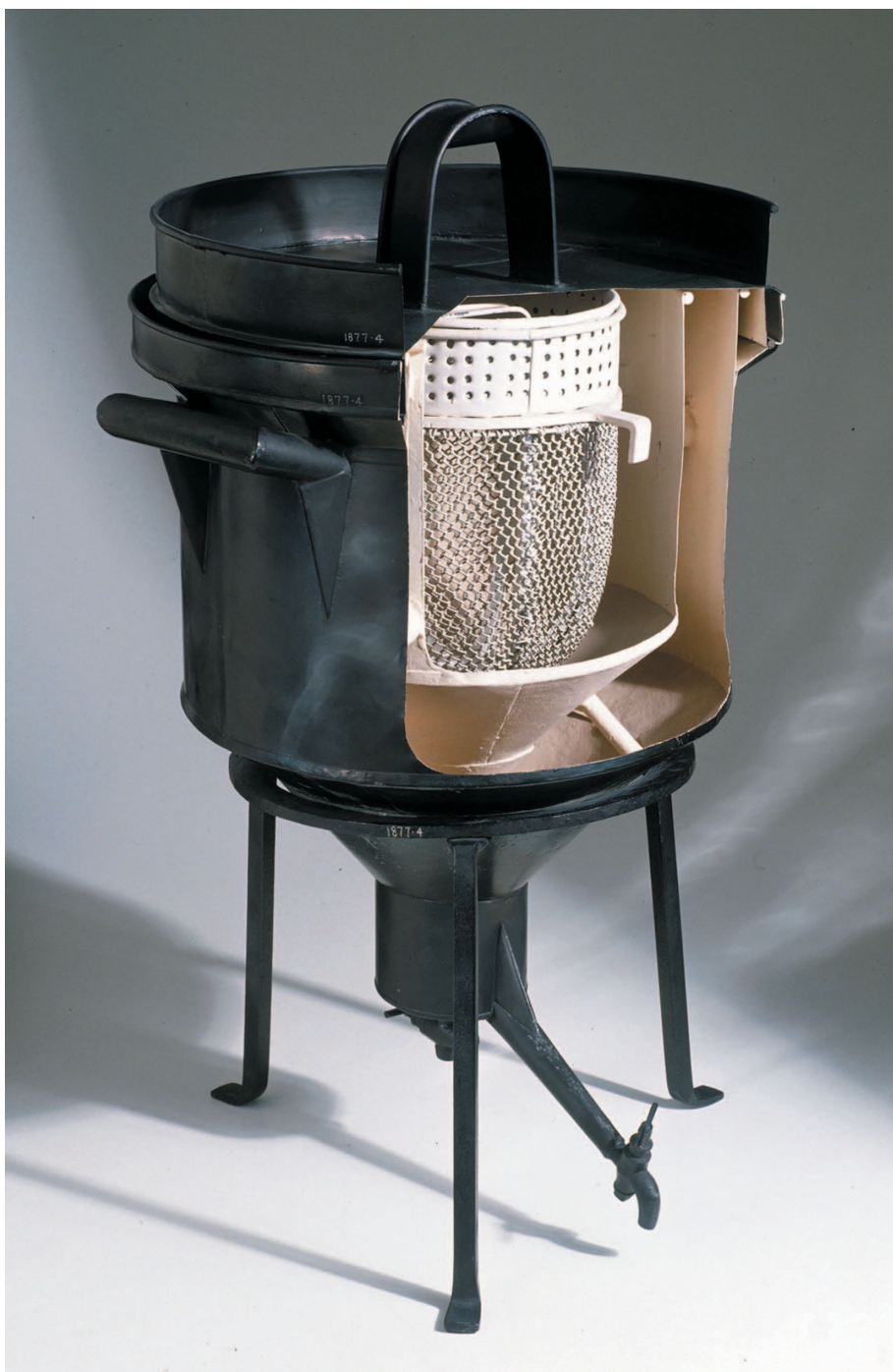
Plate 11. An exact model of Lavoisier's Ice Calorimeter, with one side cut away to show the inner workings. The guinea pig was held in the mesh cage, surrounded by ice. The water produced from ice in the inner jacket by the dissipation of metabolic heat flowed down the tube to be captured and weighed. The outer jacket was also filled with ice to minimise heat transfer between the calorimeter and the laboratory. (Image: Science Museum/Science & Society Picture Library). (see page 174)
