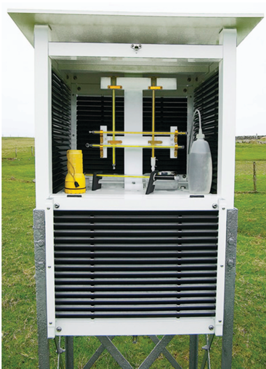
Plate 4. The interior of a modern Stevenson screen housing a range of thermometers (dry bulb and wet bulb mounted vertically, and maximum and minimum mounted horizontally). Also present are a torch to take readings by night and a water bottle to keep the wet bulb wet (Image Wikimedia Commons). (see page 47)
