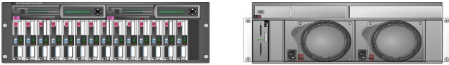
Figure 1.9 Front and back of a shared SCSI array
