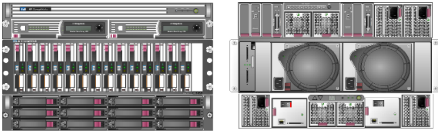
Figure 1.10 Front and back of an entry-level SAN with SATA drives
