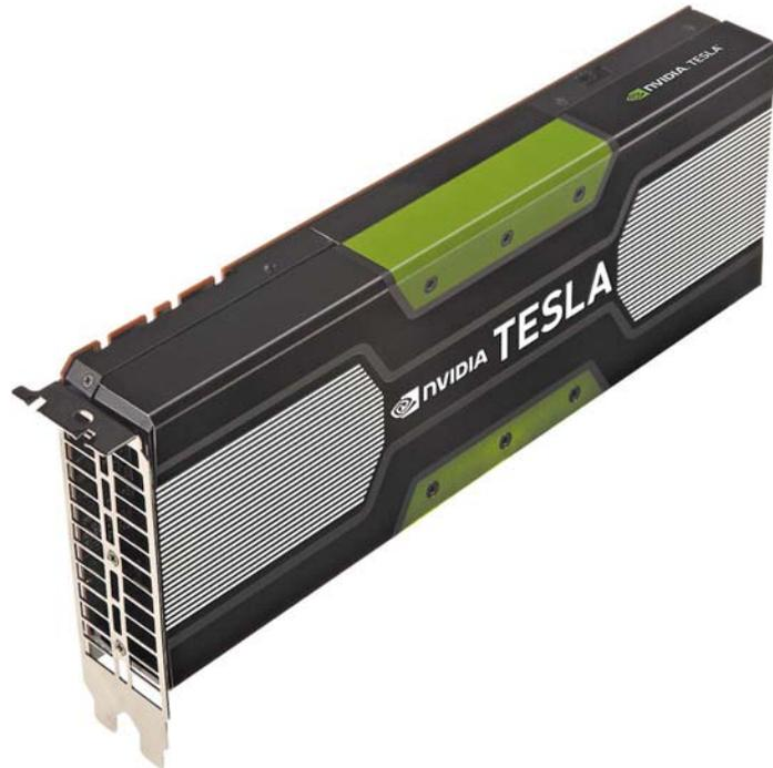
**Figure 1.23** nVidia's Tesla K20 card has 5 GB of RAM and 2496 cores.
