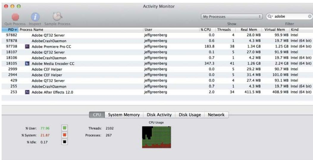
**Figure 1.27** The Activity Monitor shown here is being taxed heavily by the simultaneous use of Adobe Premiere Pro and Adobe Media Encoder.
