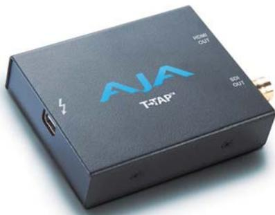
**Figure 1.26** The AJA T-Tap is one of the most inexpensive ways to perform output monitoring. Plug Thunderbolt into your system and then plug in a broadcast monitor via HDMI or HD-SDI.
