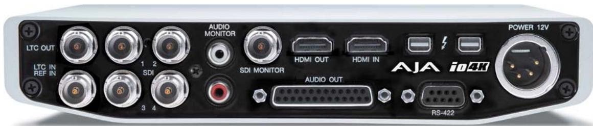
Figure 1.12 Breakout cards and boxes permit the professional evaluation of video on studio monitors (not to be confused with a regular LCD or LED flat panel). The AJA IO 4k will handle 4k and Ultra HD over Thunderbolt 2.
