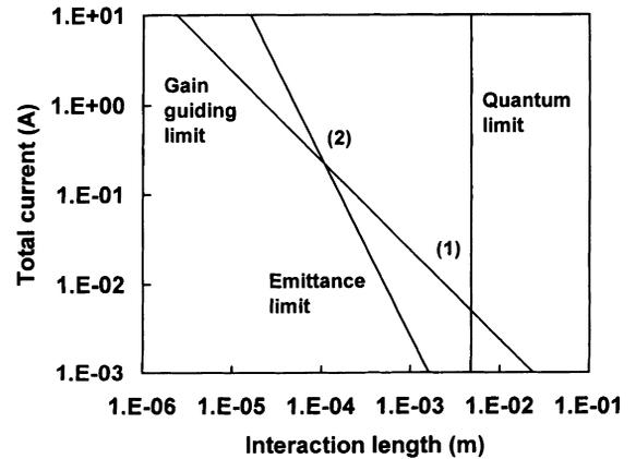
Fig. 2. Window in parameter space where a Thomson free-electron laser can be operated. The intersection labeled (1) corresponds to the maximum length and minimum current before quantum effects become important. The intersection labeled (2) corresponds to the minimum length and minimum current before emittance effects become important.
