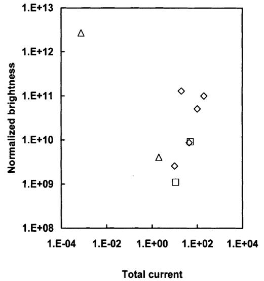
Fig. 1. Normalized brightness of various electron-beam sources used for free-electron lasers: diamonds – rf linacs; squares – storage rings; triangles – thermionic emitters.
