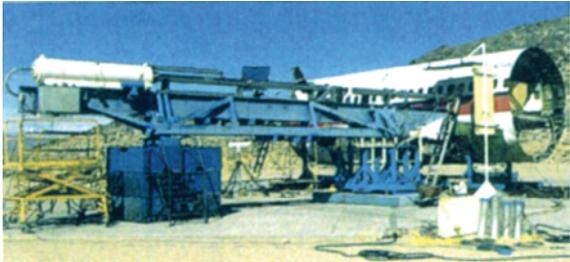
Figure 17. Full-scale testing of engine fragment barriers.
