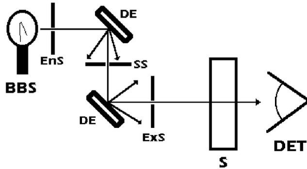
Fig. 6.1 Double-monochromator System (dispersive) optical configuration.
