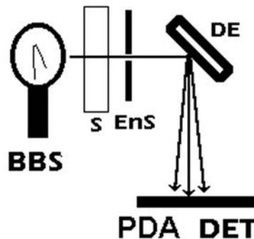
Fig. 6.3 Diode array spectrophotometer (dispersive) optical configuration.
