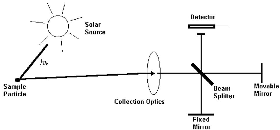
Fig. 1.4 Open-path sampling configuration using an interferometer.
