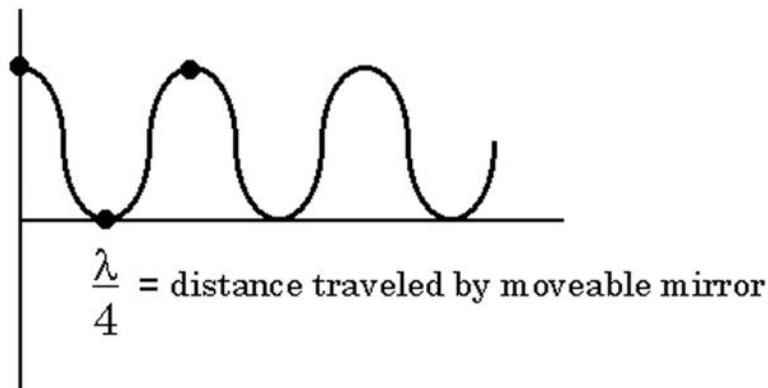
Fig. 1.7a Interferometric output as a sine wave function.
