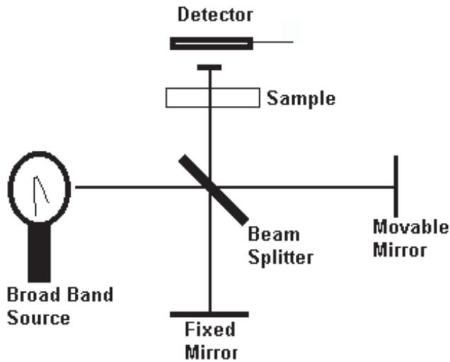
Fig. 1.3 Fourier transform spectrophotometer (interferometer) optical configuration.
