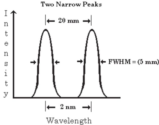
Fig. 1.11 Method to determine maximum resolution of a spectrometer under specific measurement conditions. In the example shown, Bandpass = Resolution = FWHM  $\times$  Dispersion = (2 nm) / (20 mm)  $\times$  5 mm = 0.50 nm resolution.
