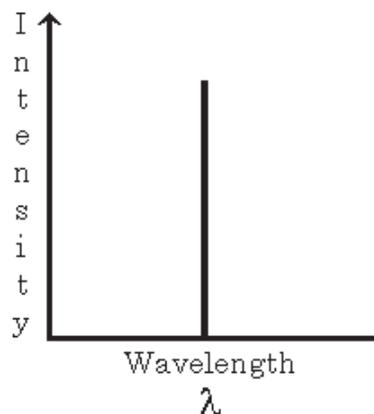
Fig. 1.8 Bright-line emission spectrum at a single wavelength as it would appear in an ideal spectrophotometer.
