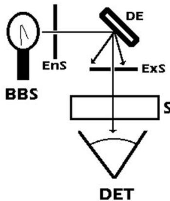
Fig. 6.2 Single-monochromator system (dispersive) optical configuration.
