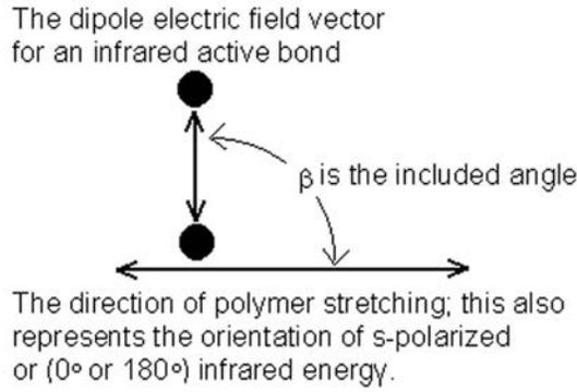
Fig. 4.1 Illustration of the bond angle between the dipole electric field vector and the direction of polymer stretching.
