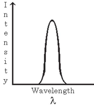
Fig. 1.9 Spectrum of a bright-line emission source (e.g., deuterium lamp). The characteristic broadening is an illustration of the bandpass of a spectrophotometer.
