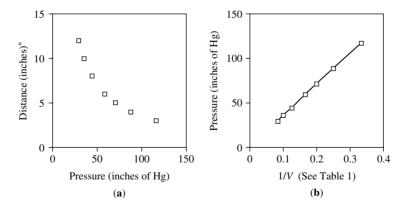
**Fig. 1** Volume of a gas (expressed as distance in a tube of constant diameter) *versus* pressure (a). Pressure as a function of reciprocal volume (b).
