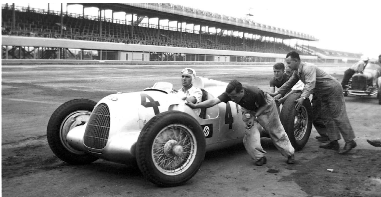
The Auto Union Grand Prix racers designed by Ferdinand Porsche had a mid-engine configuration using a supercharged V-16, and in the last Type D for 1938, a V-12. A five-speed transmission, independent suspension, and rear wheel drive with a swing axle were used for most. Mechanical specs varied, as did body shape. Aerodynamic and streamline versions were used to set land speed records. It was in one of these that German hero Bernd Rosemeyer lost his life while attempting to set a record on a German autobahn in 1938. Below he is seen taking to the track before a Grand Prix event.
