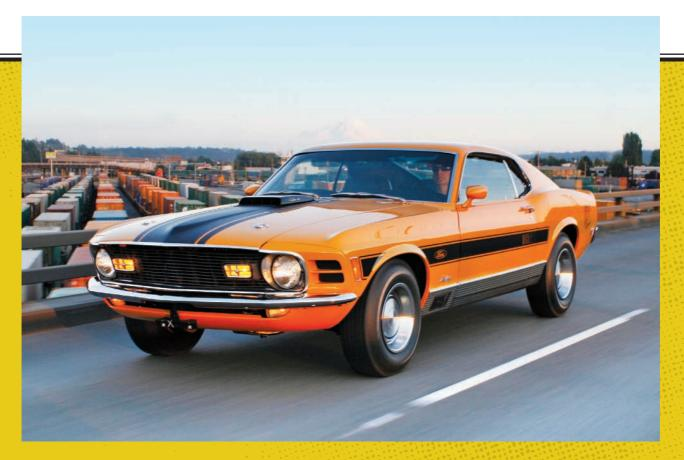
top: When powered by the stout R-Code 428 Cobra Jet, the 1970 Mach 1 came with additional heavy-duty components, including Competition Suspension and nine-inch rear axle, plus Hurst shifter and staggered rear shocks when equipped with four-speed.
