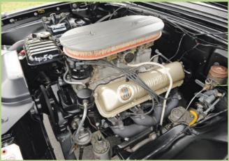
two-barrel carburetors. Rated at 401 horsepower and available in early 1961, the 6V 390 was Ford's first factory engine rated at more than 400 horsepower. The timing was critical; Ford wanted to make sure the 401 horses were legal for January's NHRA Winternationals. Many of the units were supplied in the trunk for dealer installation, but a few full-size Fords rolled off the assembly line with the six-barrel induction.
