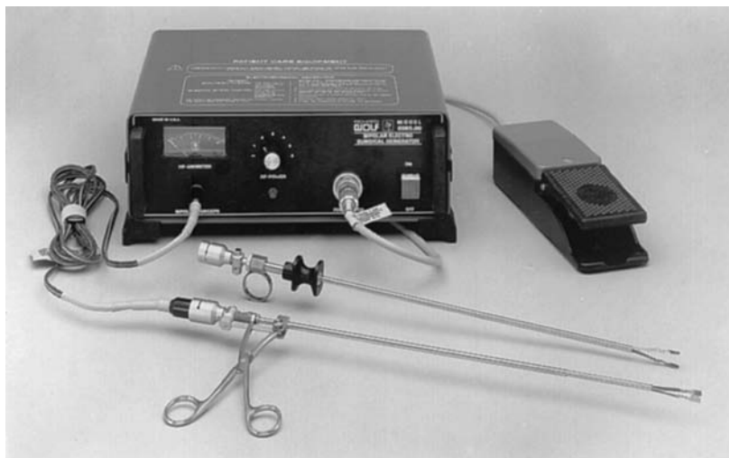
Figure 2.21. An electrogenerator with different types of bipolar forceps.
