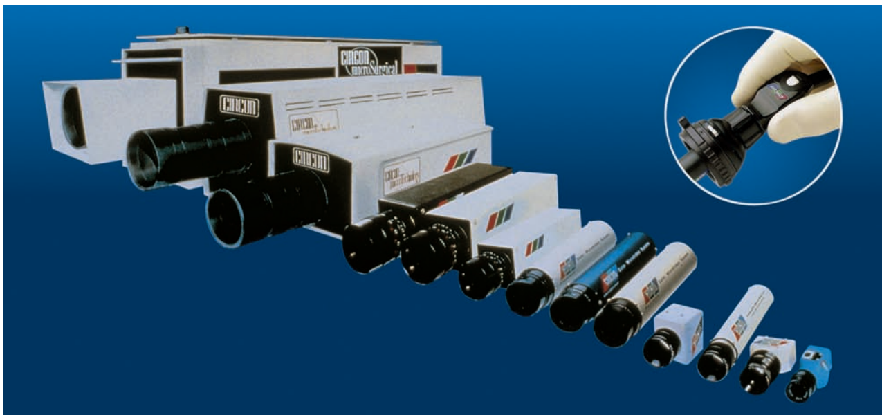
Figure 2.53. The decrease in size of video cameras over the years is illustrated. The inset shows a contemporary camera head.
