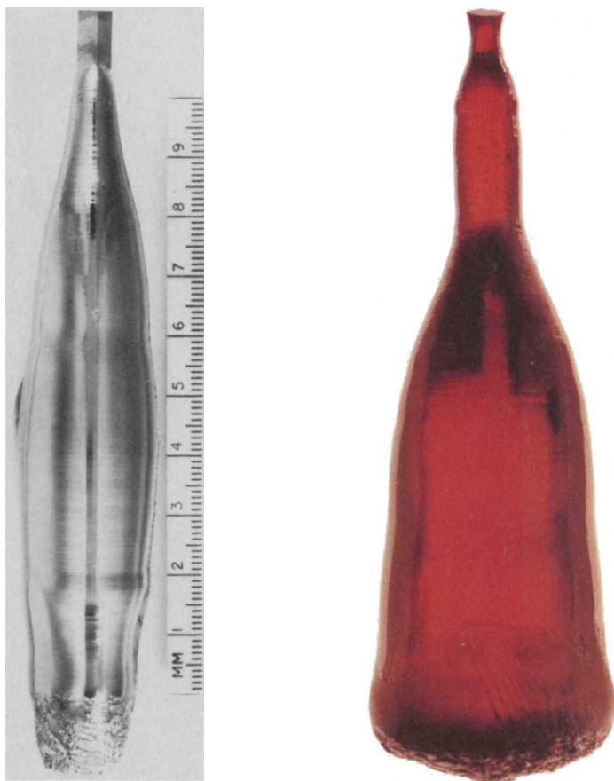
Fig. 3. Single crystals of (left) InP; (right) GaP grown by the LEC technique. Note, crystal appears red from transmitted light.
