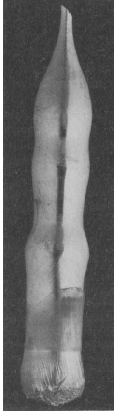
Fig. 4. LEC-GaAs crystal. The variation in crystal diameter illustrates the problem with manual control.
